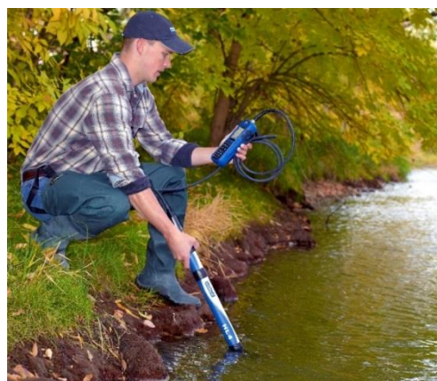
Pic. 1 Discrete monitoring of temperature, DO, pH, and Conductivity using HYDROLAB HL4
