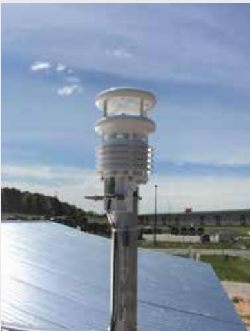
LUFFT WS500 monitoring the solar power plant in Fort Pickett. Image: Virginia National Guard
