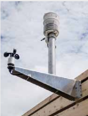
LUFFT WS800 mounted to the solar roof in Chur, Switzerland. Image: dhp technology
