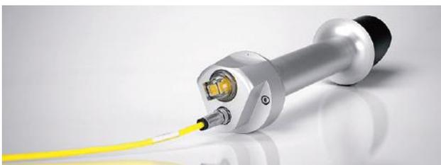
The CHP 1 Pyrliometer meets all the requirements of BSRN. It has a quartz window to provide the required spectral response range and a double-tube construction to minimise the thermal shock effects of wind and rain. There are integrated alignment aids.
