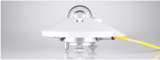
The CMP 21 and CMP 22 Pyranometers meet all the requirements of BSRN. They have high quality waterproof connectors for ease of exchange and calibration. The desiccant cartridge can be simply unscrewed and the highly accurate bubble level can be seen without removing the clip-on sun shield.
