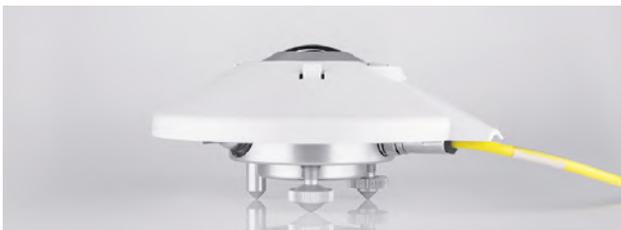
The CGR 4 Pyrgeometer meets all the requirements of BSRN and has the convenient design features of the CMP 21 and CMP 22. CGR 4 has a specially designed Silicon meniscus dome with an internal solar-blind optical filter coating and an external hard-carbon (synthetic diamond) coating. The unique thermal coupling of the dome to the housing provides the lowest thermal offsets available and no dome temperature measurement or correction is necessary.
