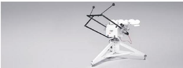
The 2AP Sun Tracker exceeds the requirements of BSRN and is widely used in measurement programmes around the world, including at Antarctic research stations.
