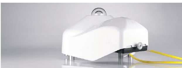
The VCV4 Ventilation Unit is specifically designed for the CMP Pyranometers and the CGR 4 Pyrgeometer. The Ventilation Unit is mounted to the Sun Tracker and then the radiometer is mounted on the VCV4 base plate. After levelling, the cover is fitted.
