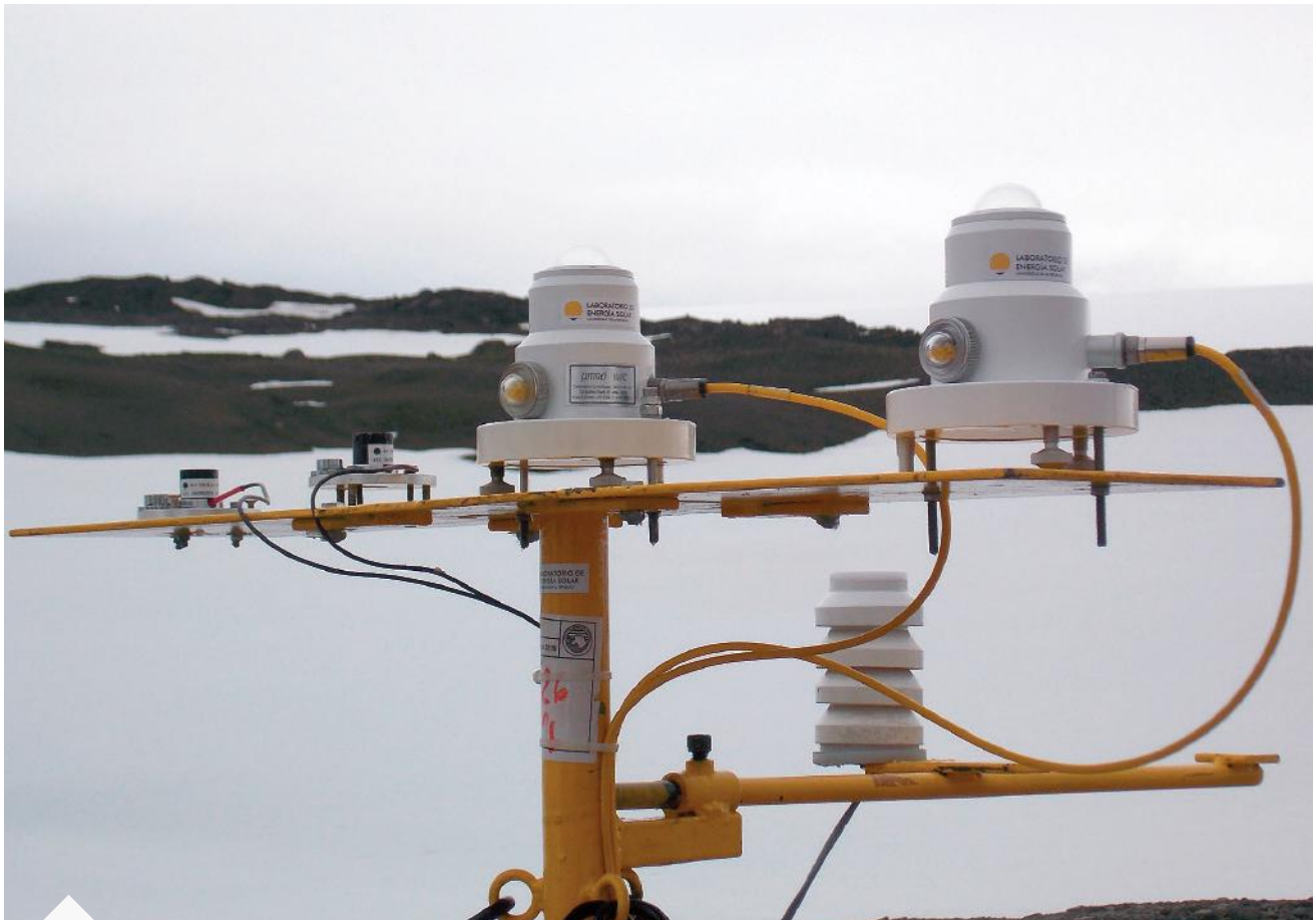
UVS radiometers at Collins Harbour in the Antarctic summer of 2016-2017
