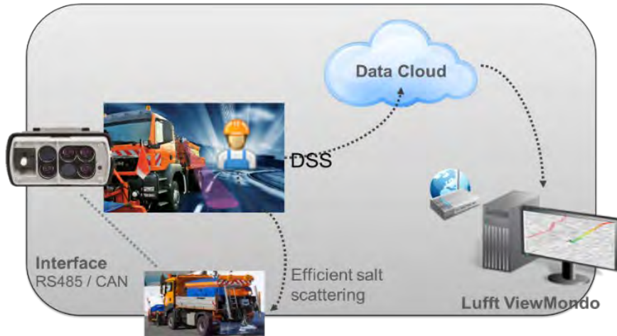
Fig. 8: Typical winter service workflow from measurement to data evaluation
