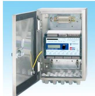
Kipp & Zonen usually supplies the COMBILOG 1020 data logger from Friedrichs in Germany (shown in the picture at right). This is easy to programme and has a built-in display and function control, performance is broadly similar to the Campbell CR 1000.
