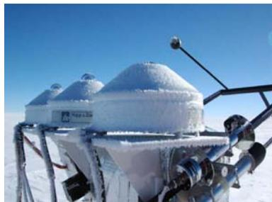
The 2AP Sun Tracker exceeds the requirements of BSRN and is widely used in measurement programmes around the world, including at Antarctic research stations.
