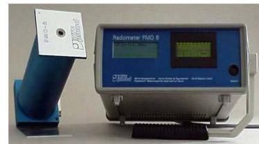
Both ACRs consist of a radiometer and a separate control unit. The PMO 6 is shown in the picture at right.
