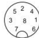
III 26: View on solder connection of the cable socket
